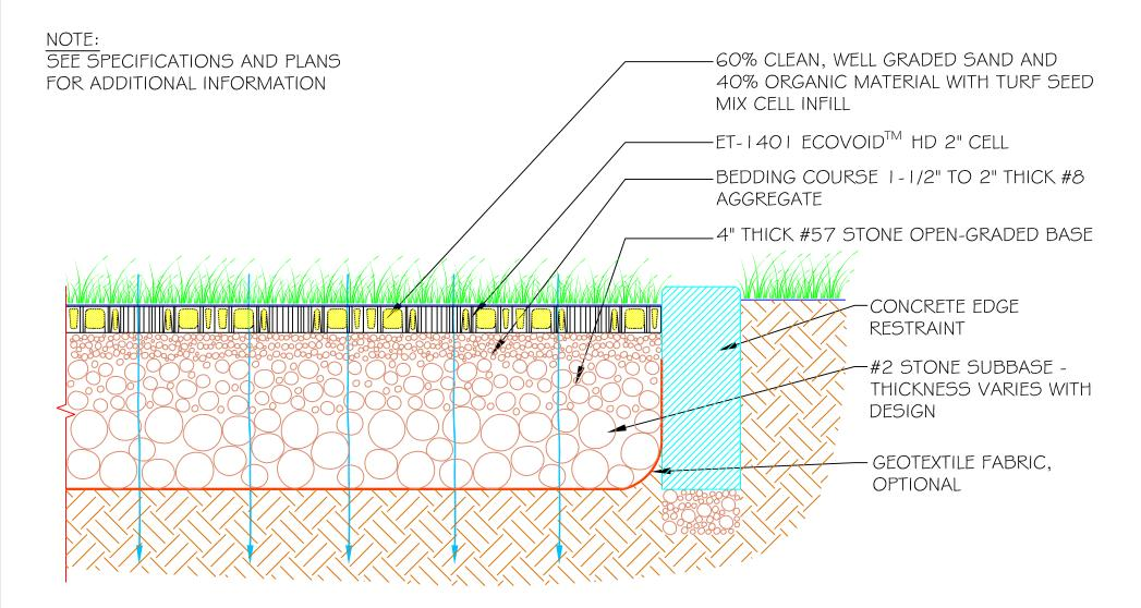
CONCEPT ECOVOID™ CELL TURF PAVER INSTALLATION SECTION - FULL EXFILTRATION
